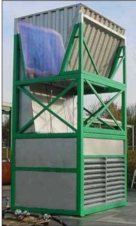
Photograph 3 – Clean Enclosed Burner
